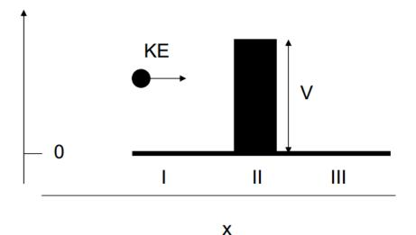
This shows 3 regions I, II and III. Here the region II is filled with a potential barrier. This has a length L and a potential V. Both I and III have zero potentials.
